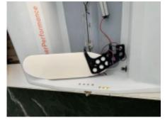
4) Tie the boat down. For 420Es, slide cradle strap through the jib lead and secure through jib cleat (just as you would with the jib sheet while sailing upwind). For FJs, slide the cradle strap through the eye below the chainplate, tighten, and secure with a double hitch.
