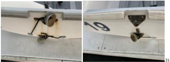
Lay rudder parallel to the stern inside the back of the boat, with rudder head on the bottom of the boat and rudder blade pointing towards the sailing center.
